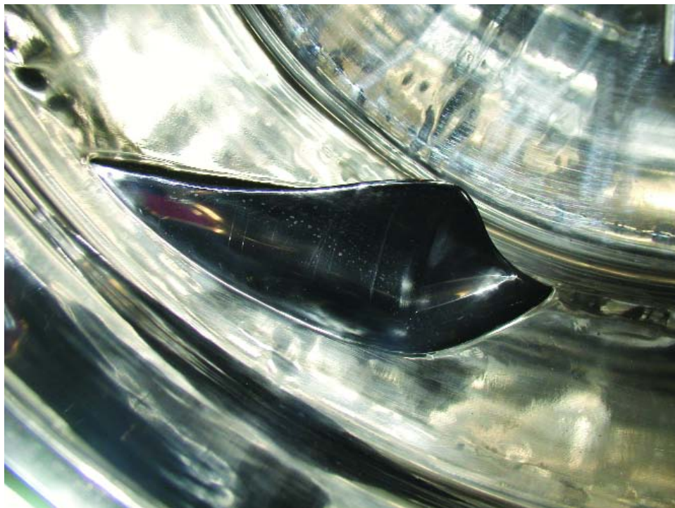
This mixing baffle [5] has a unique shape that offers gentle yet efficient mixing in a non-perforated pan.
